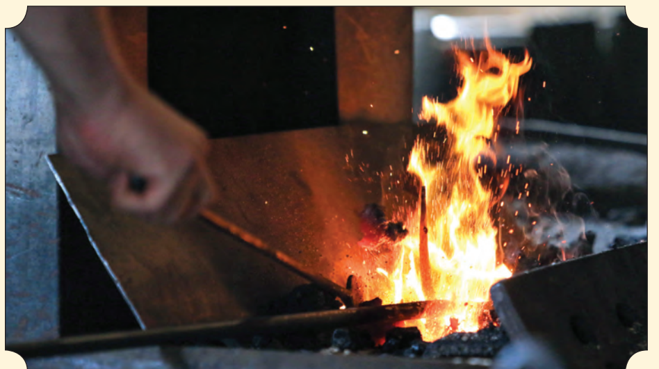
ABOVE; A rod of metal is heated up so it can be bent and molded into a firepoker.
